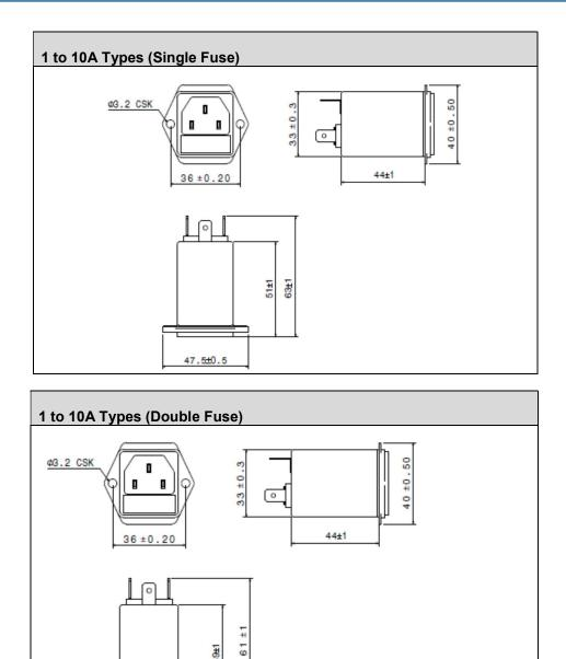
All dimensions in mm; Tolerances according to ISO2768-m
