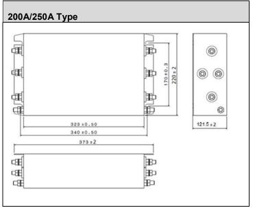
All dimensions in mm; Tolerances according to ISO2768-m
