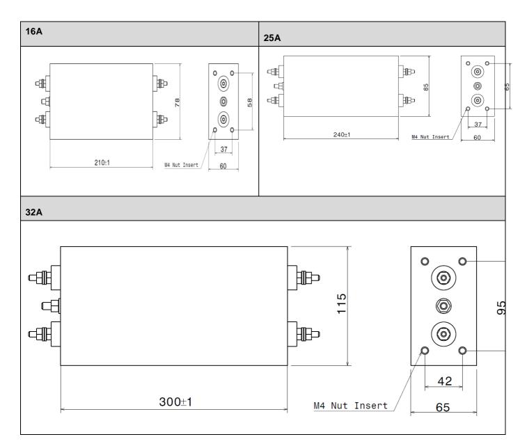
All dimensions in mm; Tolerances according: ISO2768-m
